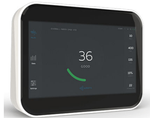
Monitors like the one shown here are being utilized to measure particulate matter, volatile compounds, carbon monoxide and dioxide, and more, informing the building system to act accordingly to maintain proper IAQ.
